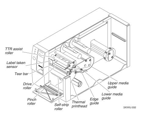
**Printer parts:** This illustration shows the printer parts that need to be cleaned. For a maintenance schedule of each part, see the Printer Maintenance Schedule table on page 32.
